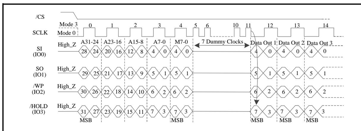
**DTR Fast Read Quad I/O with “8/16/32/64-Byte Wrap Around” in Standard SPI mode**
