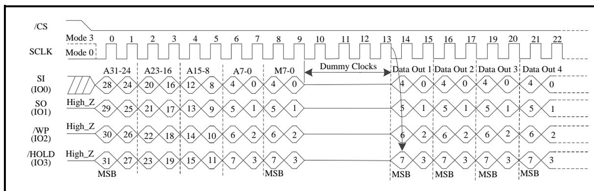
**Quad I/O Fast Read with “8/16/32/64-Byte Wrap Around”**
