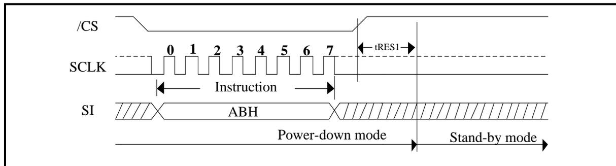
Figure 113. Release Power-Down Sequence Diagram (QPI Mode)
