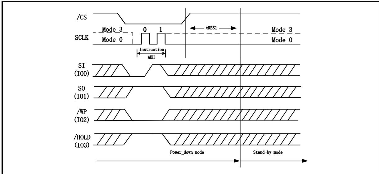
Figure 114. Release Power-Down/Read Device ID Sequence Diagram (SPI Mode)
