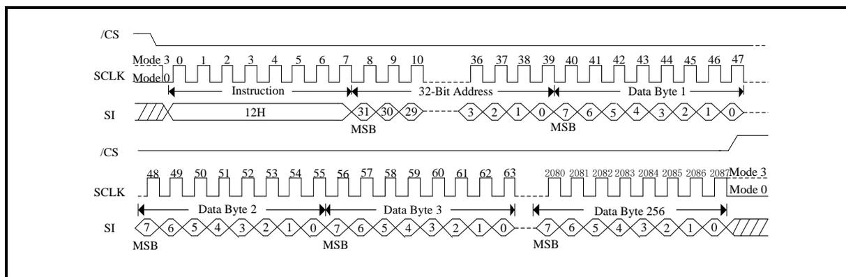
Figure 135. Page Program with 4-Byte Address (QPI Mode)
