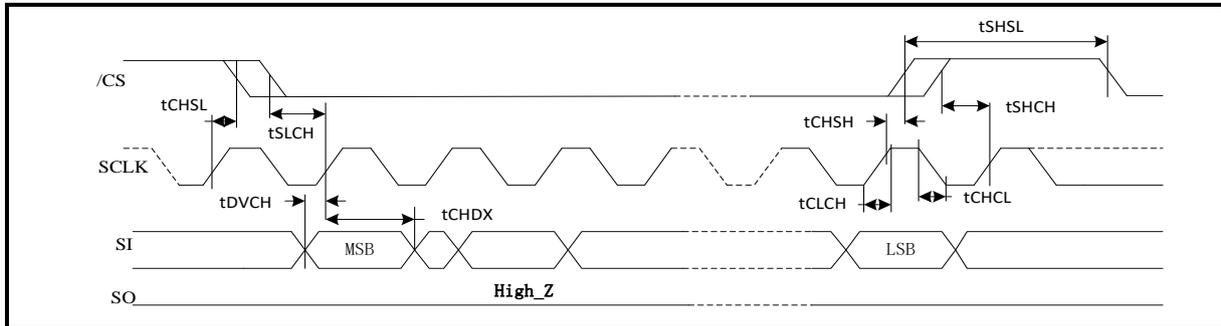
Figure 212. Output Timing
