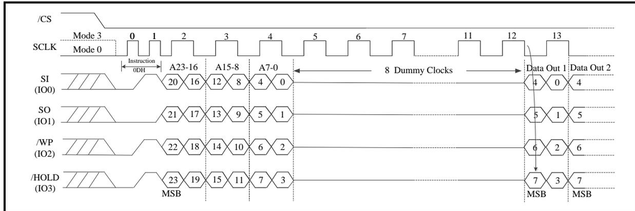
Figure 45. DTR Fast Read (QPI Mode/4-Byte Address Mode)
