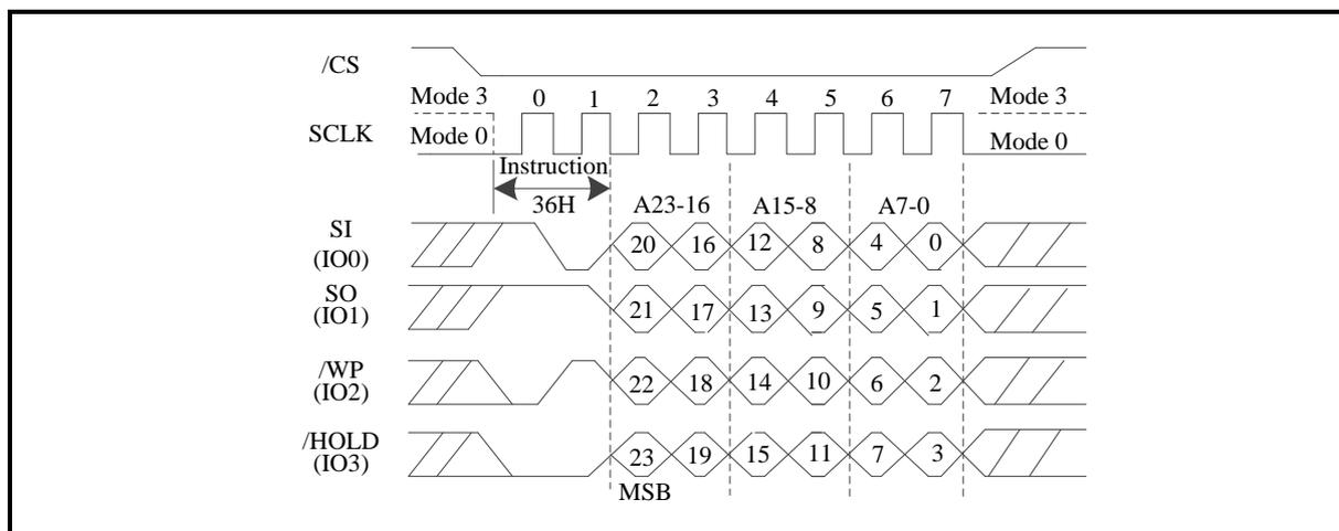
**Figure 188. Dynamic Protection Block/Sector Lock (QPI Mode/4-Byte Address Mode)**
