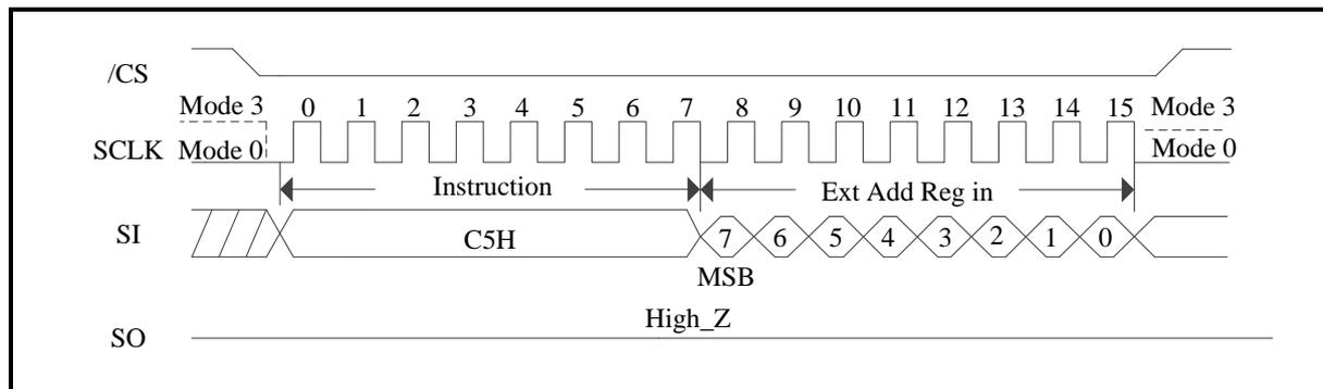
**Figure 26. Write Extended Address Register (QPI Mode)**
