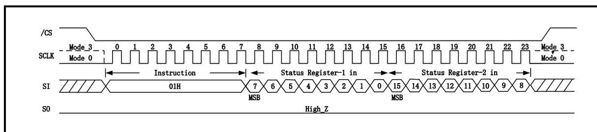
Figure 20. Write Status Register Sequence Diagram-01H 2byte (QPI Mode)
