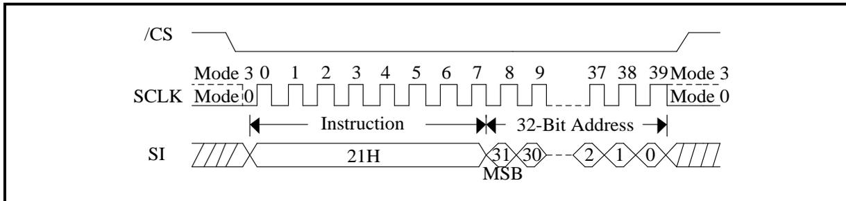
**Figure 144. Sector Erase with 4-Byte Address (QPI Mode)**
