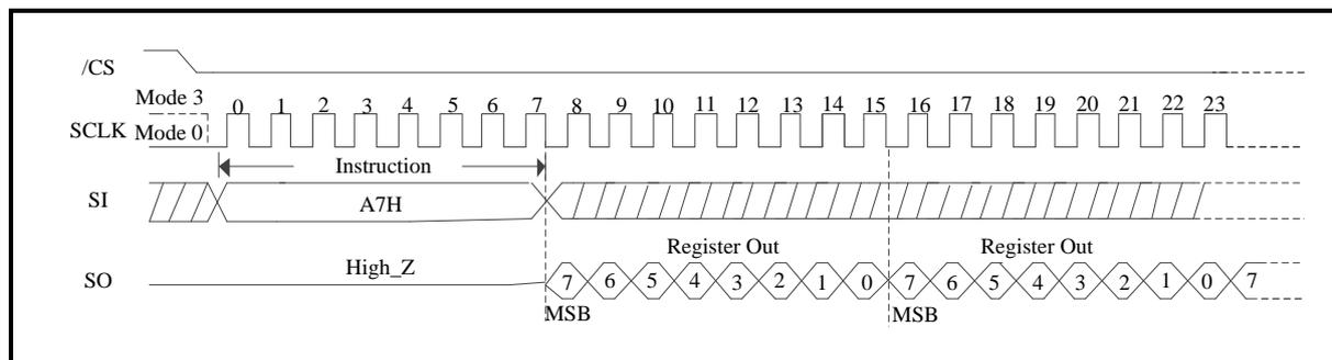
**Figure 170. Read SPB Lock Register (QPI Mode)**
