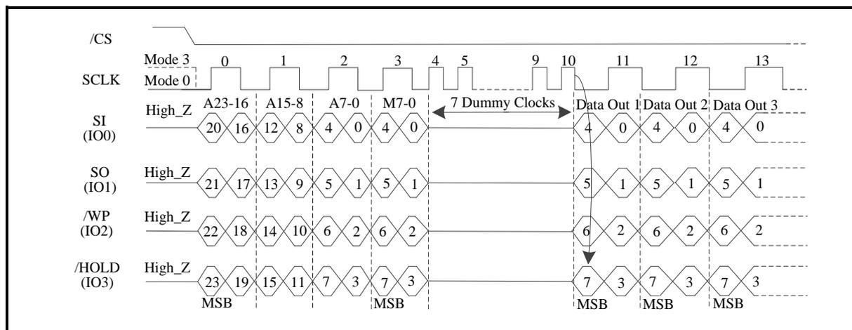
**Figure 74. DTR Fast Read Quad I/O (SPI Mode/4-Byte Address Mode; Initial instruction or previous (M5-4=(1,0)))**
