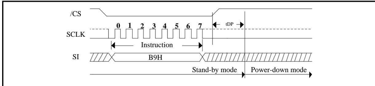
Figure 111. Deep Power-Down Sequence Diagram (QPI Mode)
