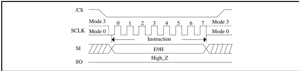
**Figure 30. Exit 4-Byte Address Mode (QPI Mode)**
