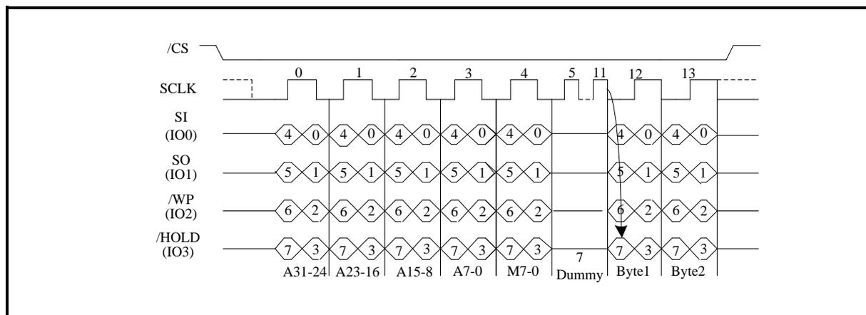
**DTR Quad I/O Fast Read with 4- Byte Address with “8/16/32/64-Byte Wrap Around” in Standard SPI mode**
