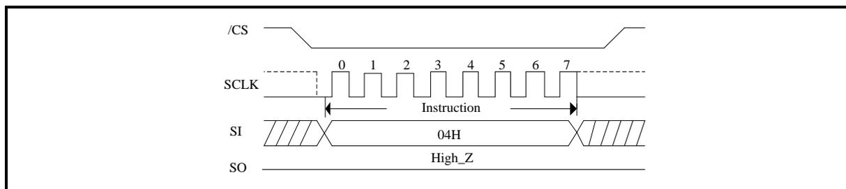
**Figure 16. Write Disable Sequence Diagram (QPI Mode)**
