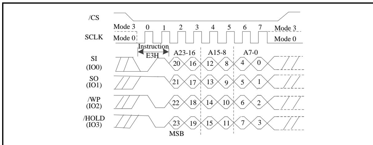
Figure 178. SPB Program (QPI Mode/4-Byte Address Mode)
