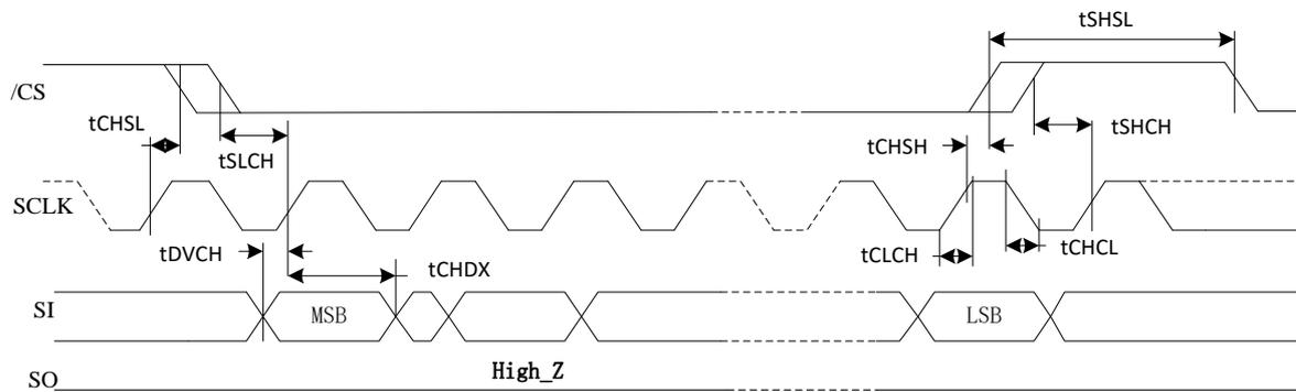
Figure 38. Output Timing
