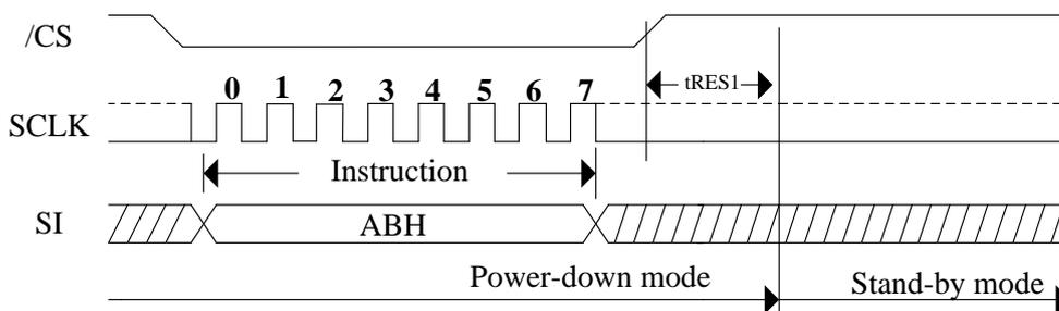
Figure 14b. Release Power-Down/Read Device ID Sequence Diagram
