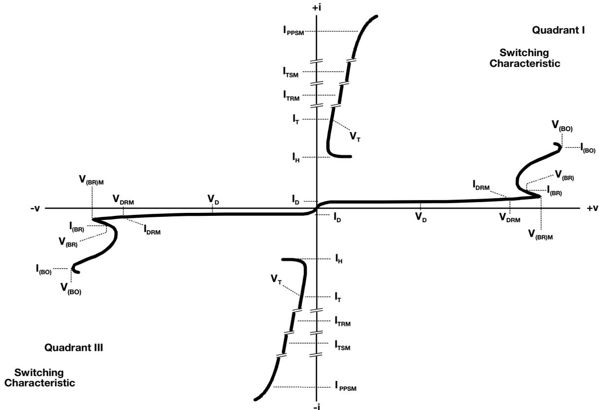
Figure 1. Voltage-Current Characteristic for the Ring and Tip Terminals
