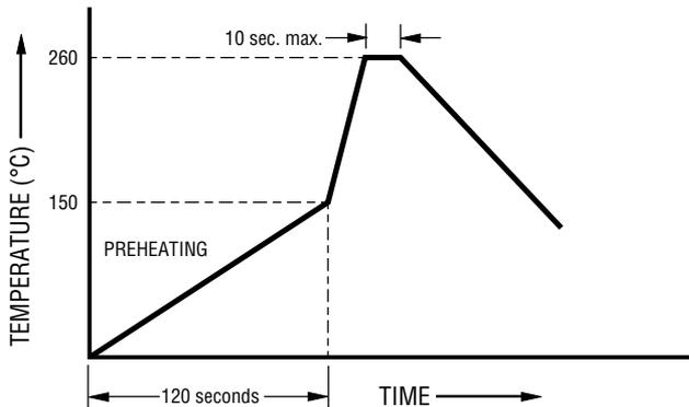
Wave soldering is suitable for 2410 size models.
