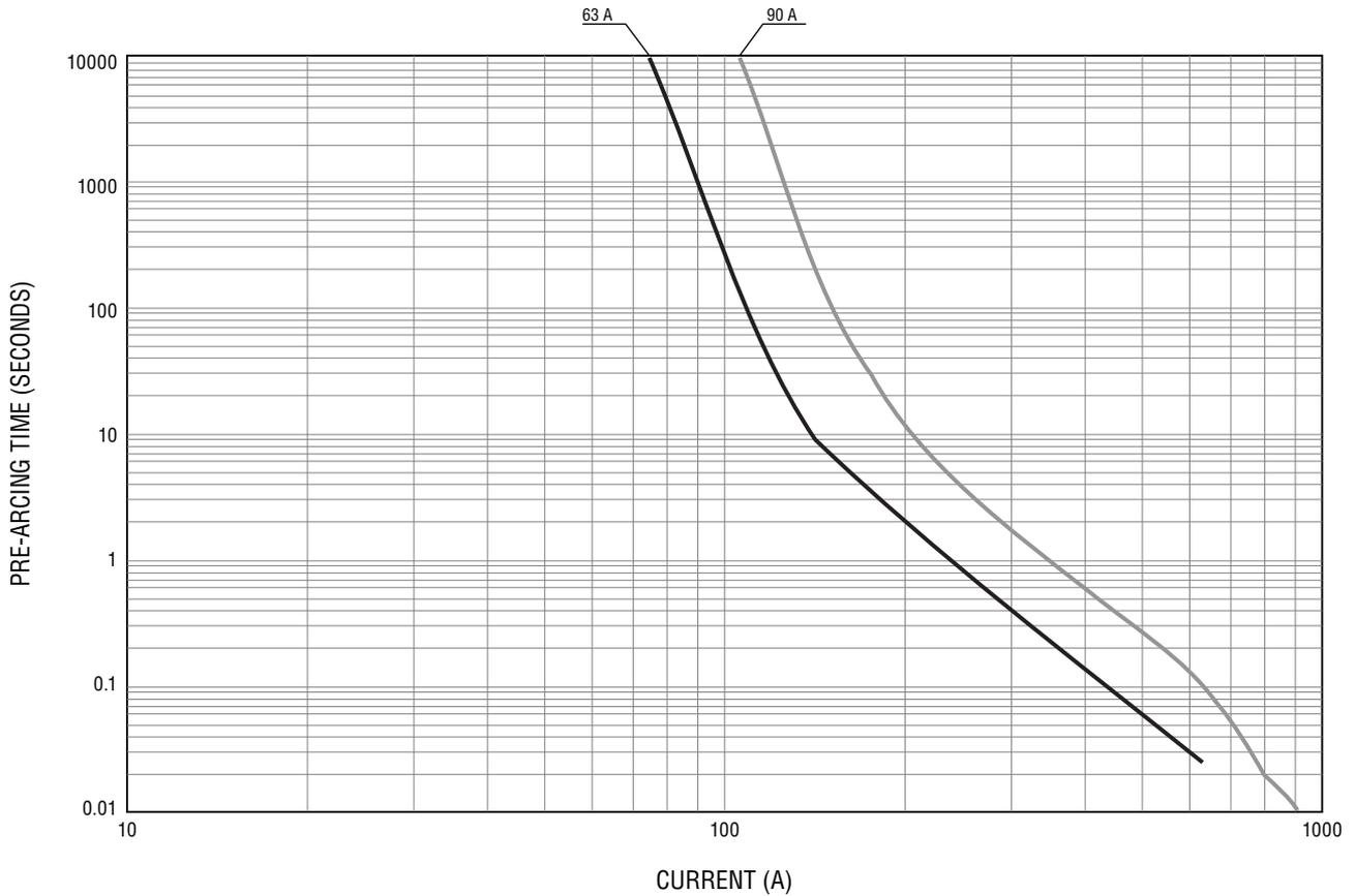
Current Rating Thermal Derating Curve
