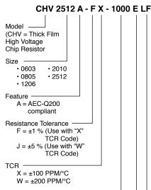
Resistance Value 1 % Tolerance: First three digits are significant, fourth digit represents
