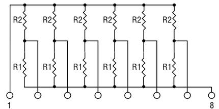
The 4608X-104 (shown above) is an 8-pin configuration and terminates 6 lines. Pins 1 and 8 are common for ground and power, respectively. Twelve thick-film resistors are paired in series between the common lines (pins 1 and 8).
