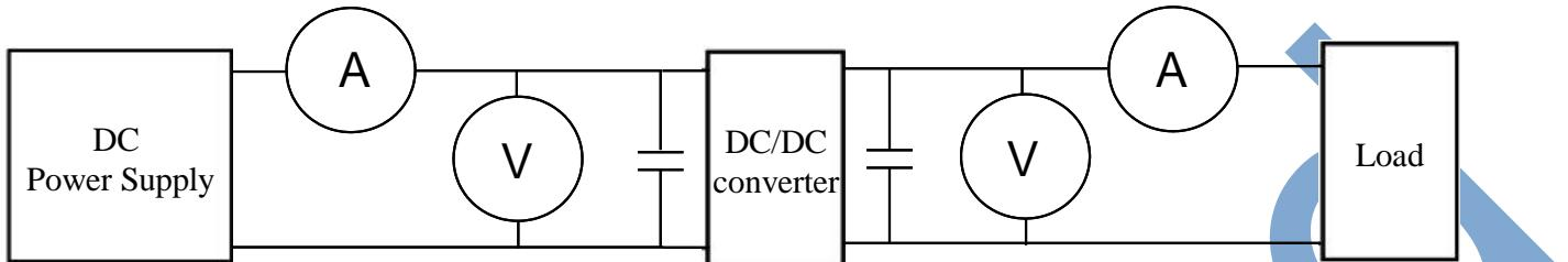
◎DC Power Supply: It offers a wide voltage and current range precisely.
