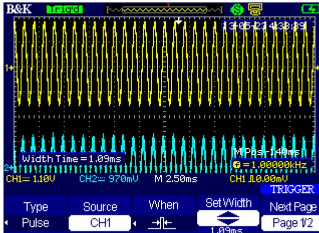
Figure 36 - Pulse Width Trigger Condition Display
