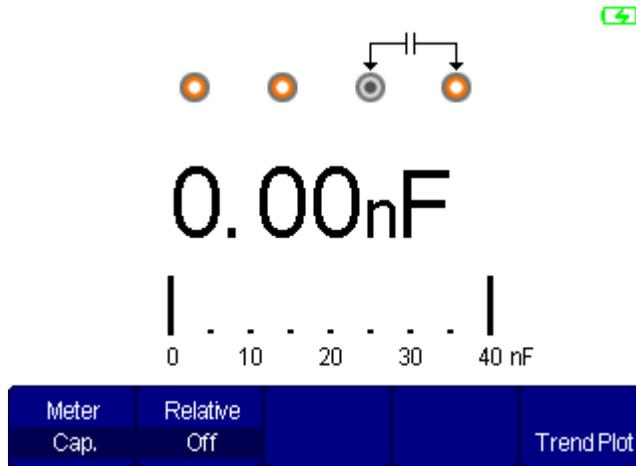
Figure 70 - Capacitance Measurement
