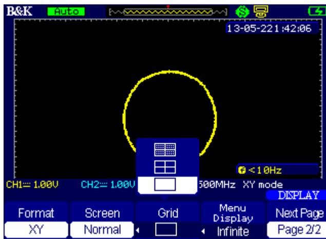
Figure 20 - No Grid and Axes Display
