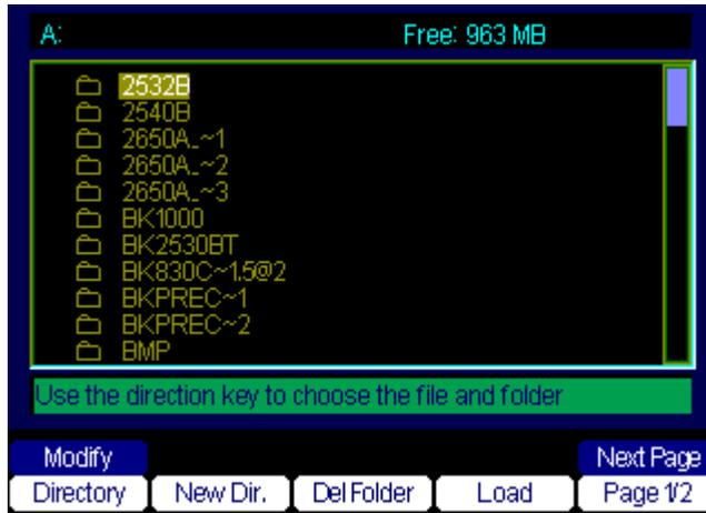
3. Follow the same instructions from section “3.7 Save/Recall Function” to create a directory and/or a new file, then select **Load** from the menu to save all recorded data into a new file on the external USB flash drive.
