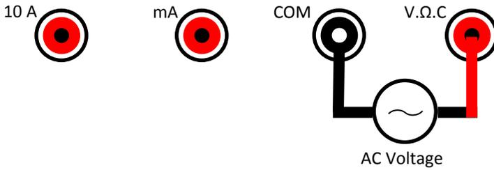
Figure 61 - Connection for AC Voltage Measurement
