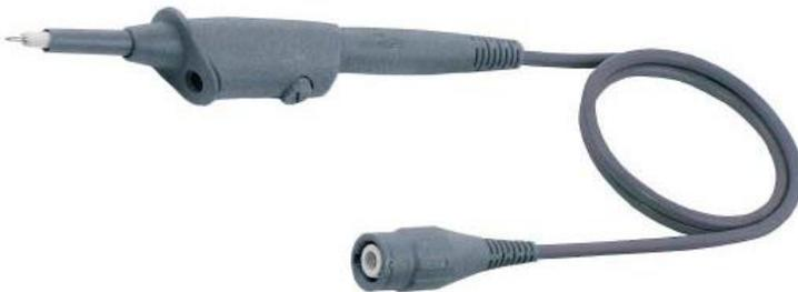
Models 2511 and 2512 come with two passive 1X/10X probes (PR150SA) with the following specifications:
