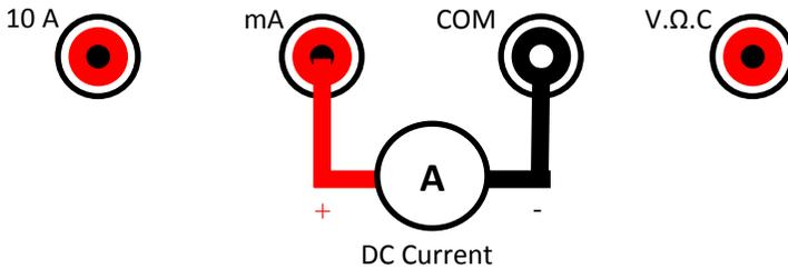
Figure 62 - Connection for Low DC Current Measurement
