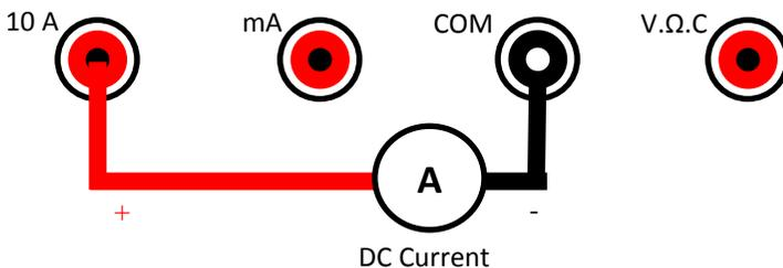
Figure 63 - Connection for Higher DC Current Measurement
