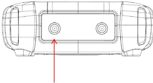
3. Attach the probe compensation connector to the miniUSB port on the side of the instrument.
