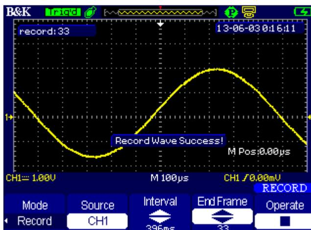
Figure 48 - Recording Finished
