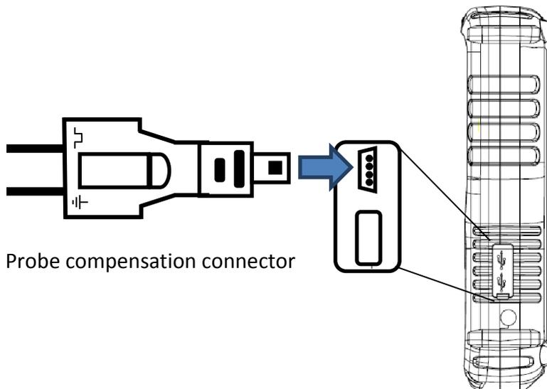
4. Connect the probe tip to the 3V port (1 kHz, 3Vpp Square Wave) and the reference ground clip to the ground port on the probe compensation connector.
