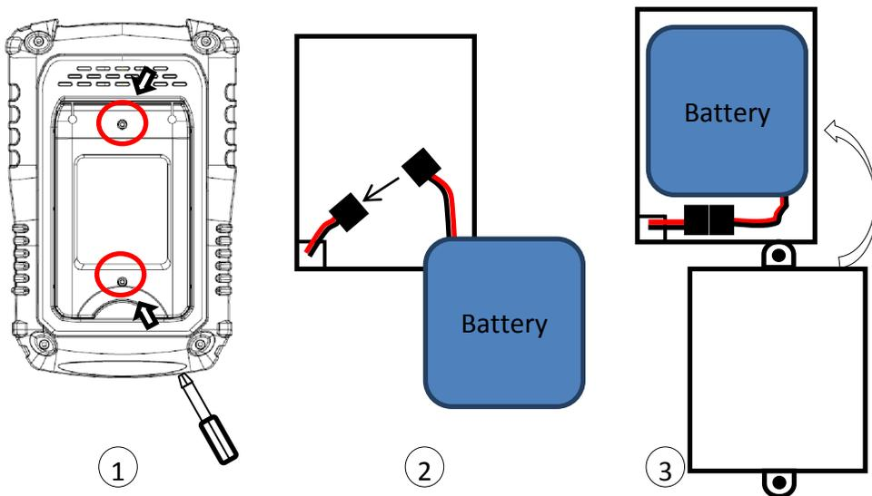
**Figure 9 - Installing Battery**
