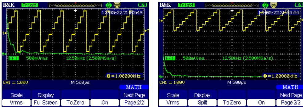
Figure 22 - FFT Full Screen (left), Split Screen (right)
