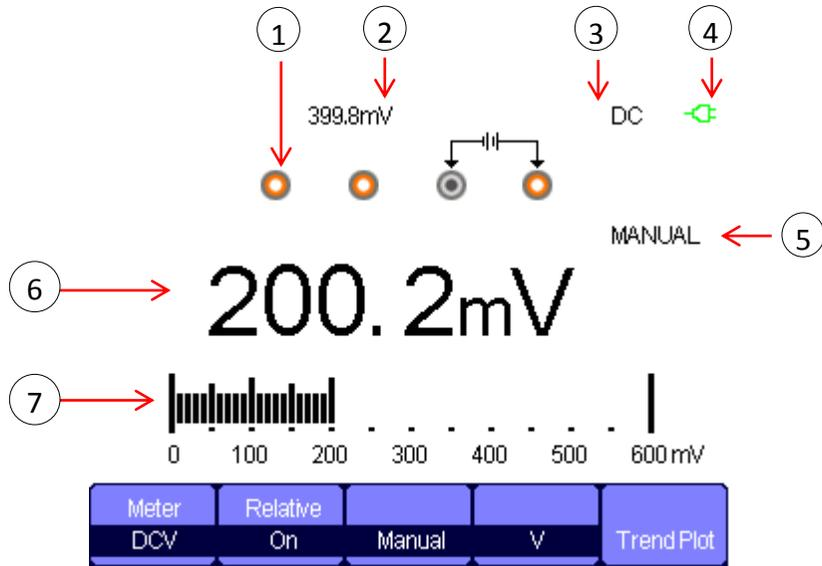
Figure 6 - Multimeter Display
