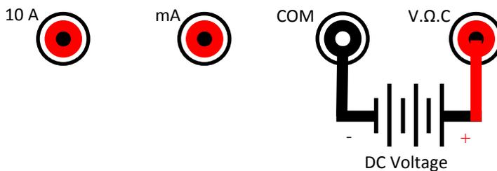
Figure 60 - Connection for DC Voltage Measurement
