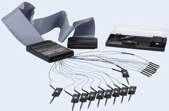
The 16-channel color-coded logic probe consists of two eight-channel pods. To make contact with the DUT, the probe connects directly to square pins or clips to test points using the included grabbers. With an input capacitance of only 8 pF and 100 kΩ input impedance, the probe protects the integrity of your signal. The probe is included with MSO models.
