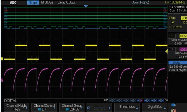
The 16 integrated digital channels are displayed along-side analog channels allowing users to view up to 18 time-correlated channels with shared triggering and acquisition on one screen. The LA2540C license enables the 16 digital channels of the 2540C Series and is included with MSO models.
