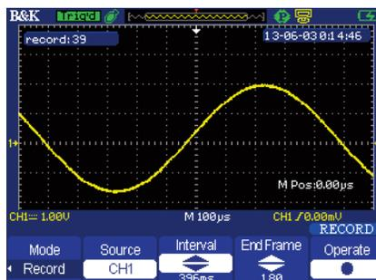
Monitor and analyze long-term signal behavior by recording data continuously over a period of time. These modes allow recorded data to be played back for post acquisition analysis.
