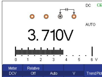
Speed up troubleshooting with the built-in 6000-count multimeter. Measurement functions include AC/DC voltage and current, resistance, capacitance, diode, and continuity test.
