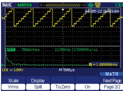
Display and measure the input signal's frequency spectrum. Select one of the 4 FFT windows: Rectangular, Hanning, Hamming, and Blackman. Use cursors to measure the spectral component's magnitude and frequency.
