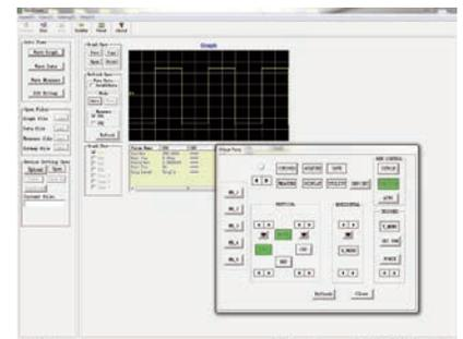
PC software provided (free download from [www.bkprecision.com](http://www.bkprecision.com)) for seamless integration between the oscilloscope and PC. Capture and transfer waveforms, screen images, setups and measurement results to a Windows PC via the USB device port on the side of the instrument. A USB host port is also available for quick and easy screen saving.
