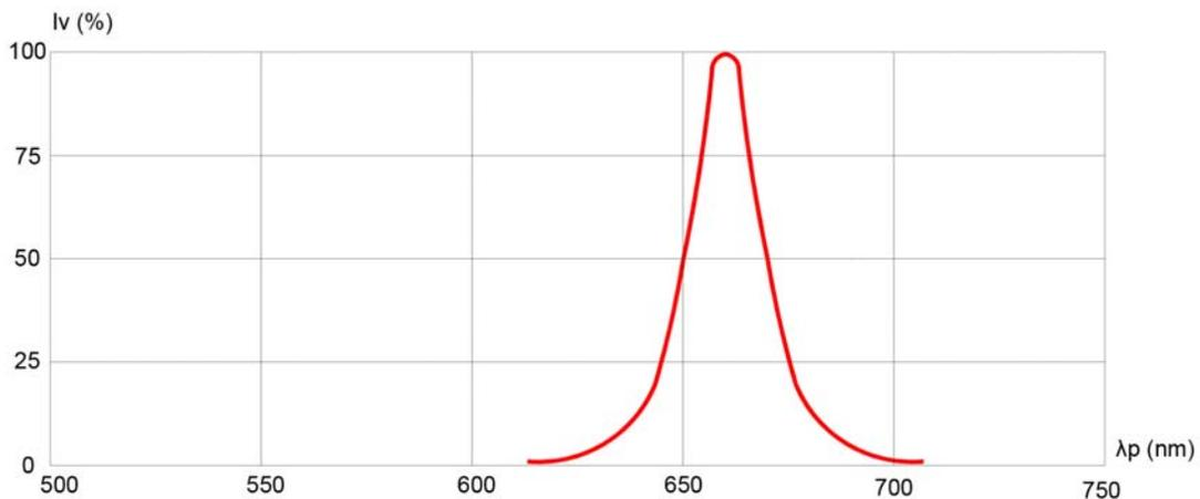
Fig. 5 Relative Luminous Intensity vs. Peak Wavelength
