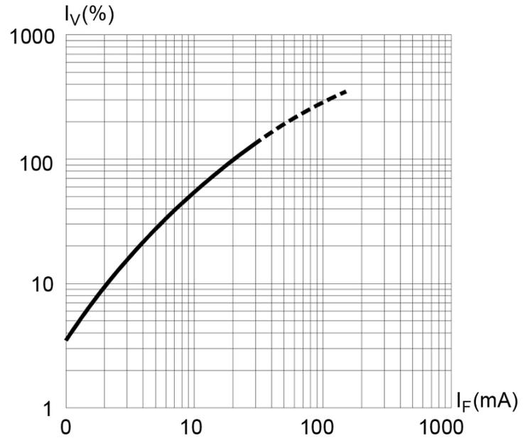
Fig. 3 Relative Luminous Intensity vs. Forward Current
