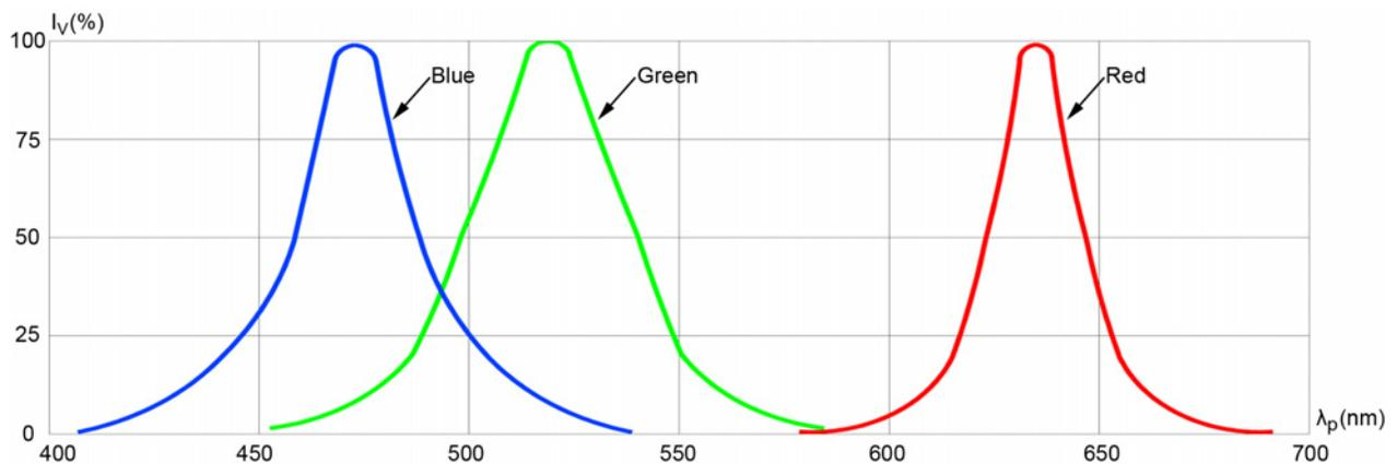
Fig. 1 Relative Luminous Intensity vs. Peak Wavelength
