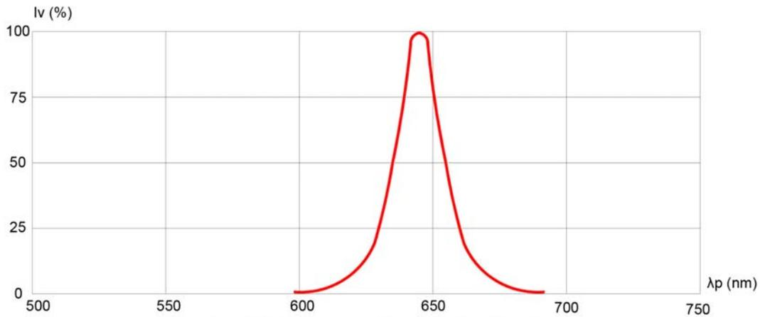
Fig. 5 Relative Luminous Intensity vs. Peak Wavelength
