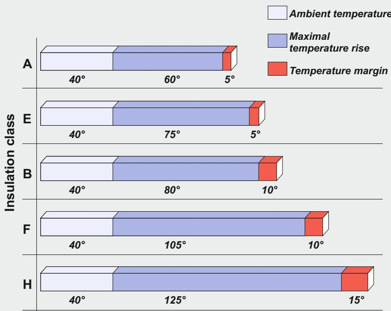
*Insulation class F for an electric motor means that at ambient temperature of 40°C the temperature rise of its windings may be max. 105°C with the additional temperature margin of 10°C (under specified measuring conditions in accordance with the IEC 60034-1 standard).*
