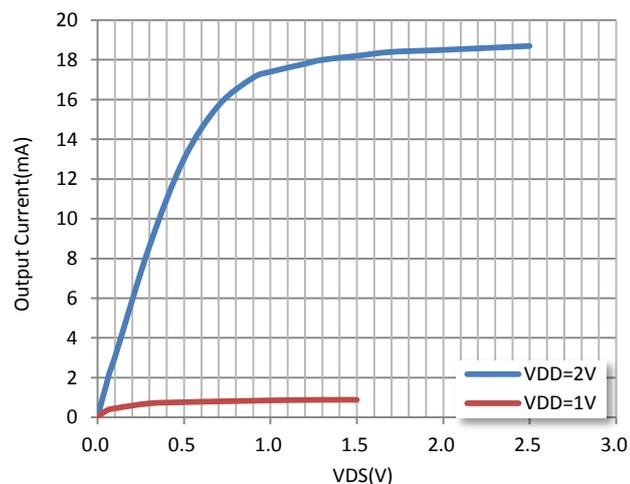
4) NCH Driver Output Current vs. Input Voltage
