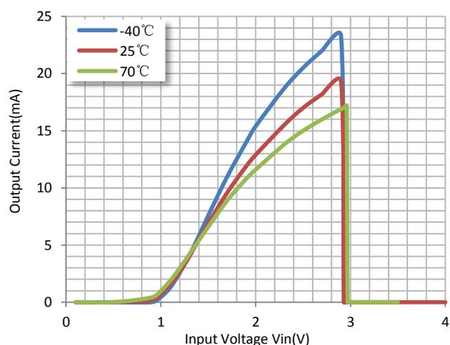
5) PCH Driver Output Current vs. Input Current
