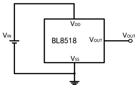
(3) NCH Drive Output Current Test Circuit
