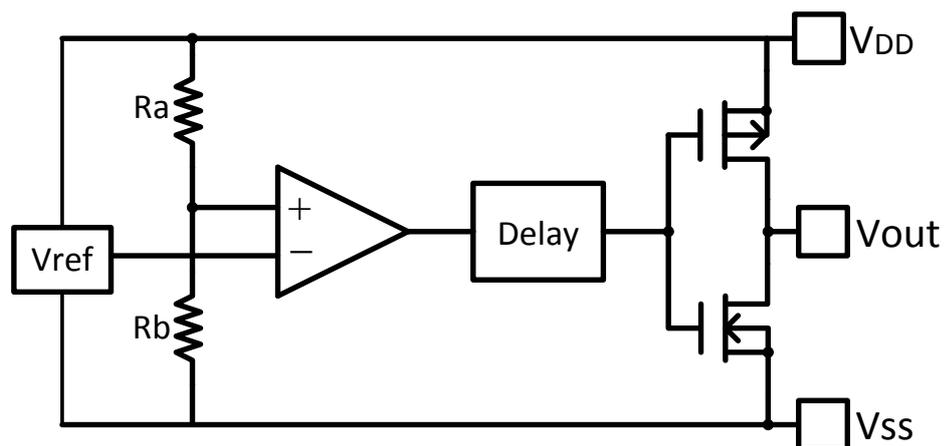
High precision low temperature co-efficiency reference voltage is applied to the negative input of a comparator. Input voltage, divided by resistor array of Ra and Rb, is applied to the positive input of the comparator. Output of the comparator passes a delay circuit and a series of buffer to drive the output CMOS pair.
