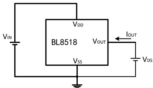
(4) PCH Drive Output Current Test Circuit
