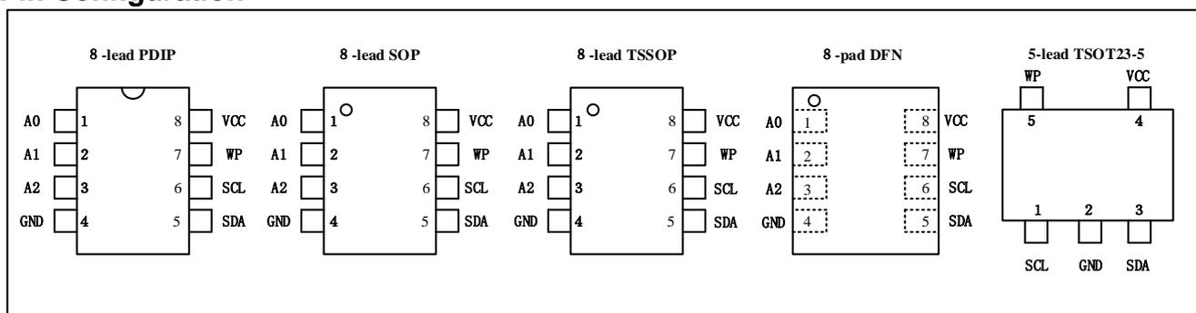
DEVICE/PAGE ADDRESSES (A2, A1 and A0): The A2, A1 and A0 pins are device address inputs that are hard wire for the BL24C64A. Eight 64K devices may be addressed on a single bus system (device addressing is discussed in detail under the Device Addressing section).
