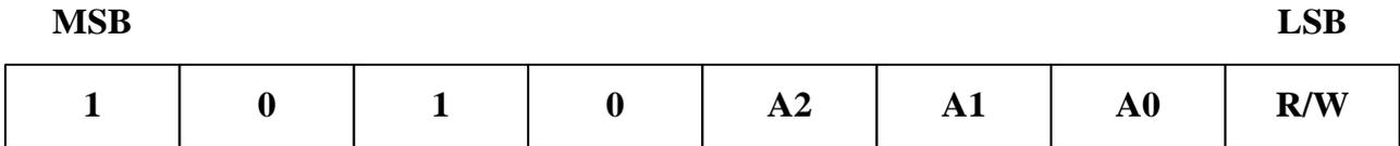
**Figure 5. Device Address**
