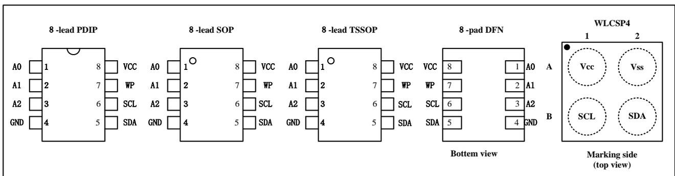
**DEVICE/PAGE ADDRESSES (A2, A1 and A0):** The A2, A1 and A0 pins are device address inputs that are hard wire for the BL24C32A. Eight 32K devices may be addressed on a single bus system (device addressing is discussed in detail under the Device Addressing section).
