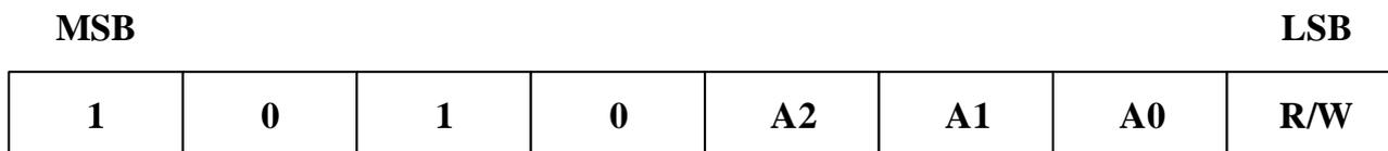
**Figure 5: Device Address**
