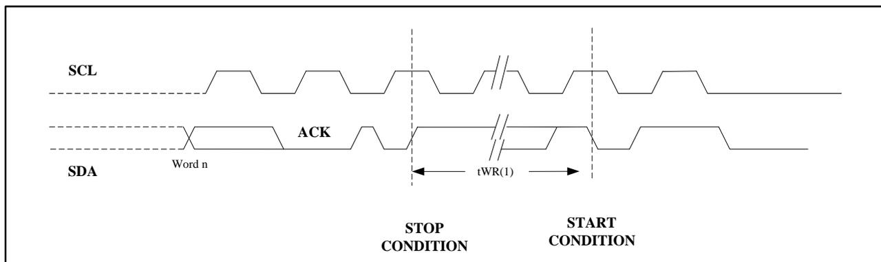
**Figure 12. SCL: Serial Clock, SDA: Serial Data I/O**
