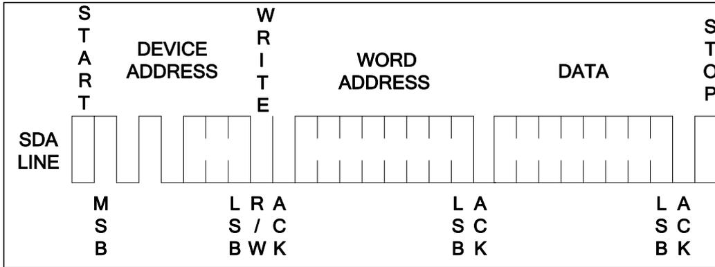
Figure 6. Byte Write
