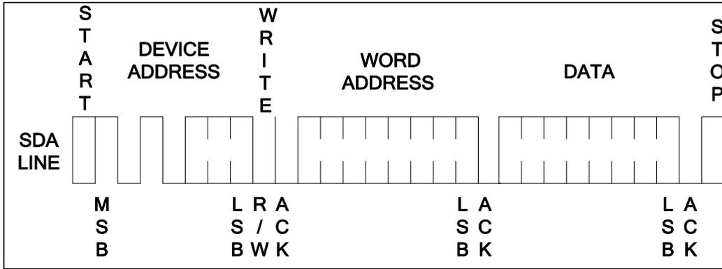
Figure 6. Byte Write
