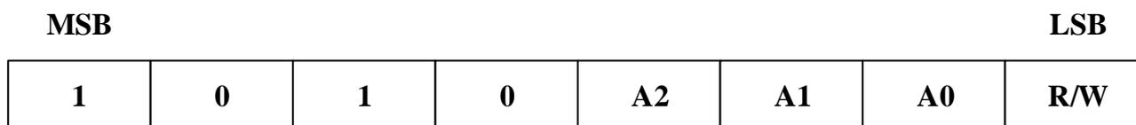
**Figure 5: Device Address**
