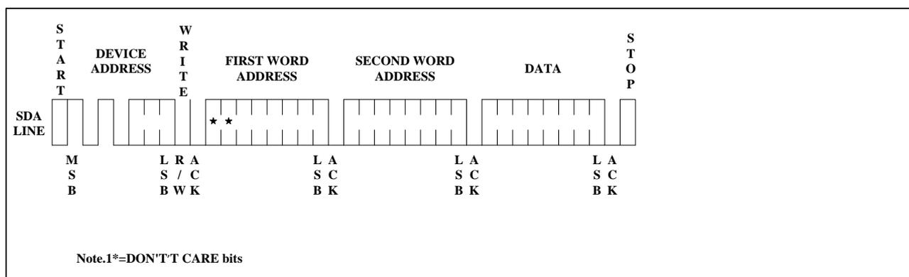
**Figure 6: Byte Write**
