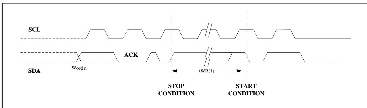
**Figure 13. SCL: Serial Clock, SDA: Serial Data I/O**
