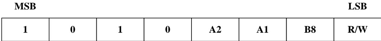
**Figure 5. Device Address**
