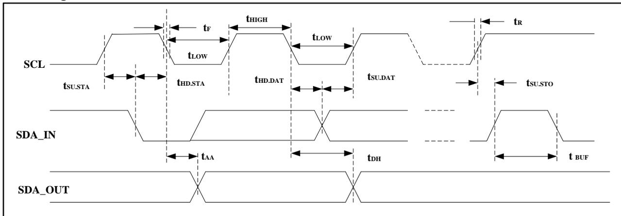
Figure 12. SCL: Serial Clock, SDA: Serial Data I/O
