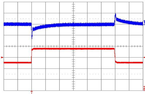
**Fig. 11:** Output voltage response to load current step-change (12.5 A – 18.75 A – 12.5 A) at  $V_{in} = 48\text{ V}$ . Top trace: output voltage (100 mV/div.). Bottom trace: load current (5 A/div). Current slew rate: 1 A/ $\mu\text{s}$ .  $C_o = 470\ \mu\text{F}$  tantalum + 1  $\mu\text{F}$  ceramic. Time scale: 0.2 ms/div.
