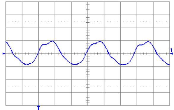
**Fig. 12:** Output voltage ripple (20 mV/div.) at full rated load current into a resistive load with  $C_o = 10\ \mu\text{F}$  tantalum + 1  $\mu\text{F}$  ceramic and  $V_{in} = 48\text{ V}$ . Time scale: 1  $\mu\text{s}$ /div.
