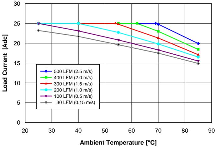
**Fig. 1:** Available load current vs. ambient air temperature and airflow rates for **QM48T25050** converter with B height pins mounted vertically with air flowing from pin 3 to pin 1, MOSFET temperature  $\leq 120^{\circ}\text{C}$ ,  $V_{in} = 48\text{ V}$ .
