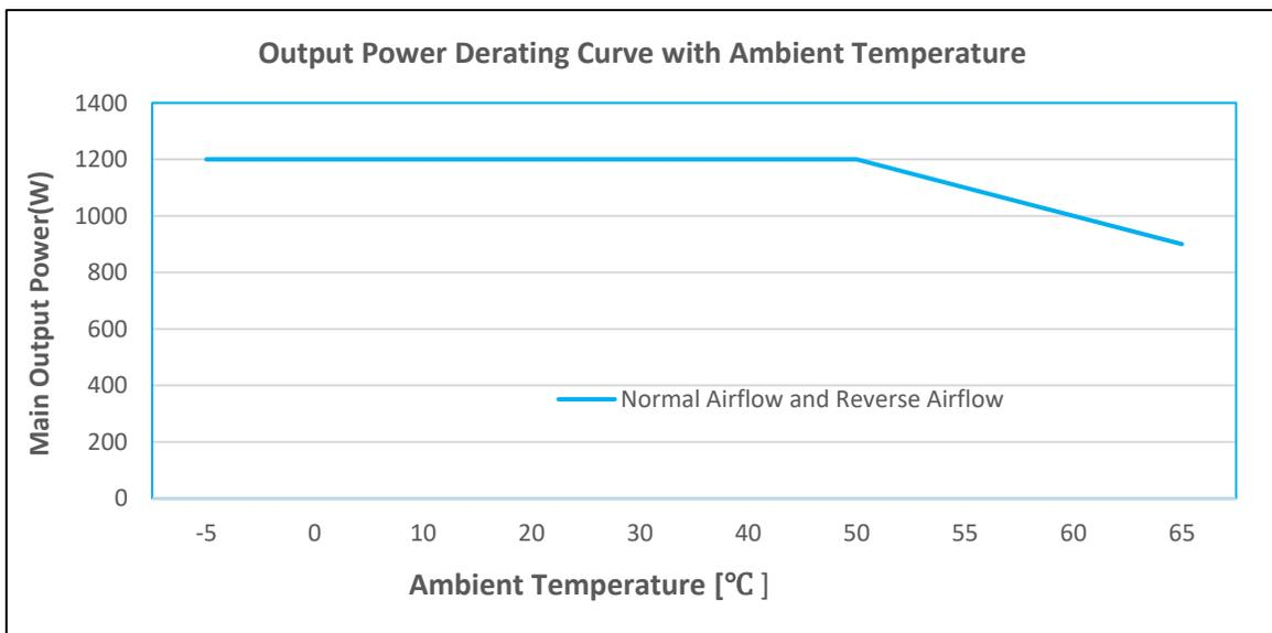
Figure 8. Derating Curve for ambient above 50°C
