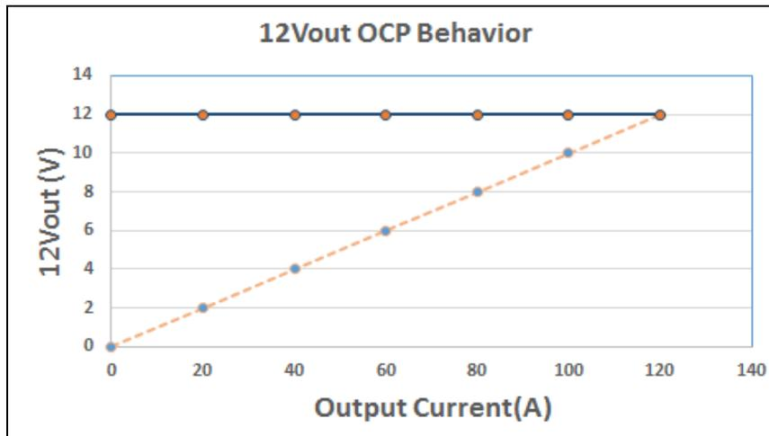
Figure 7. Current Limitation on V1
