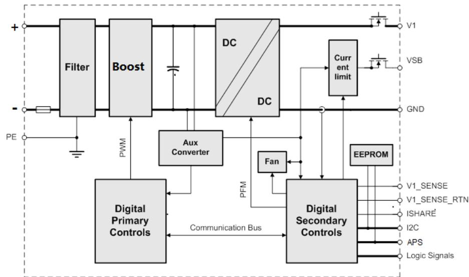
Figure 1. Block Diagram
