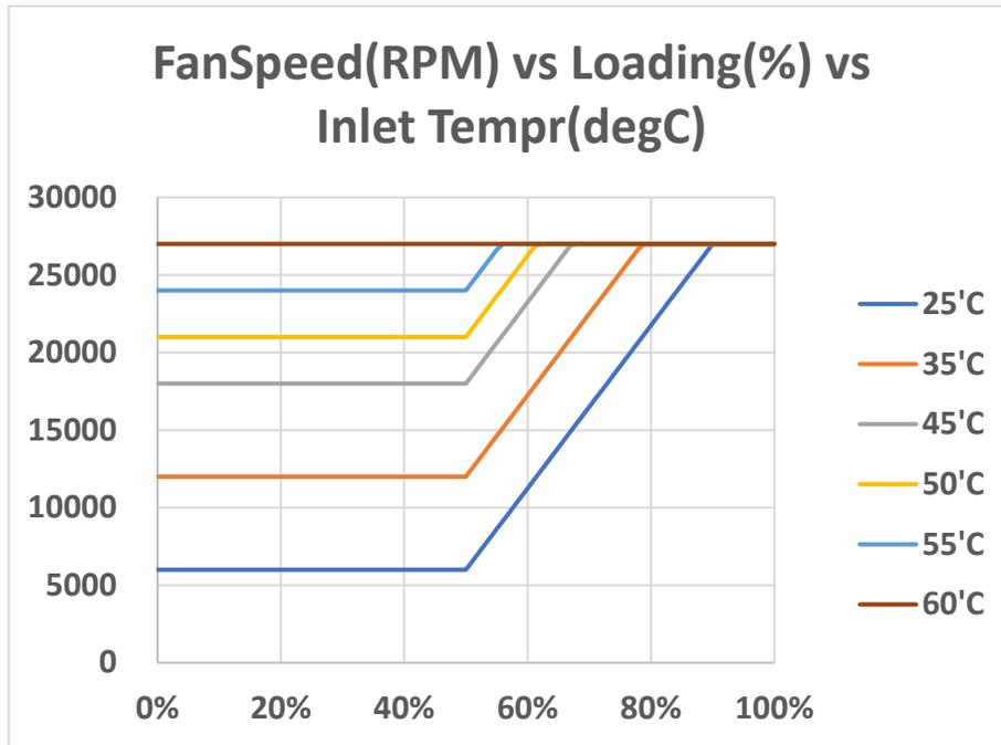
Figure 22. Fan speed vs. main output load
