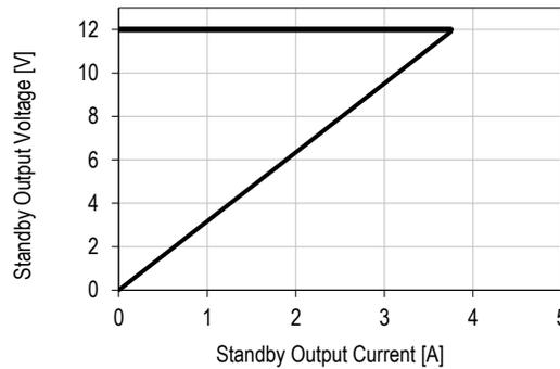
Figure 10. Current Limitation on 12 V<sub>SB</sub>
