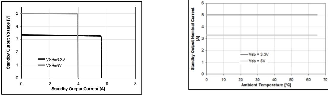
Figure 9. Current Limitation and Temperature Derating on 3.3 / 5 V<sub>SB</sub>
