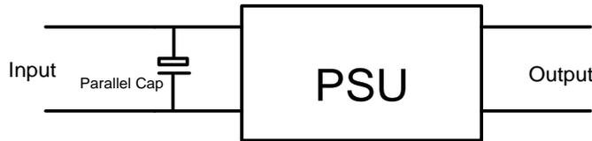
Figure 3. Parallel Cap parallel with input connector
