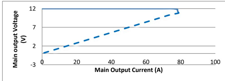
Figure 4. Current Limitation on V1 ( $V_i = 230$  VAC)
