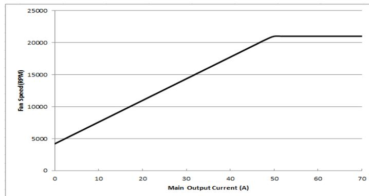
Figure 13. Fan speed vs. main output load
