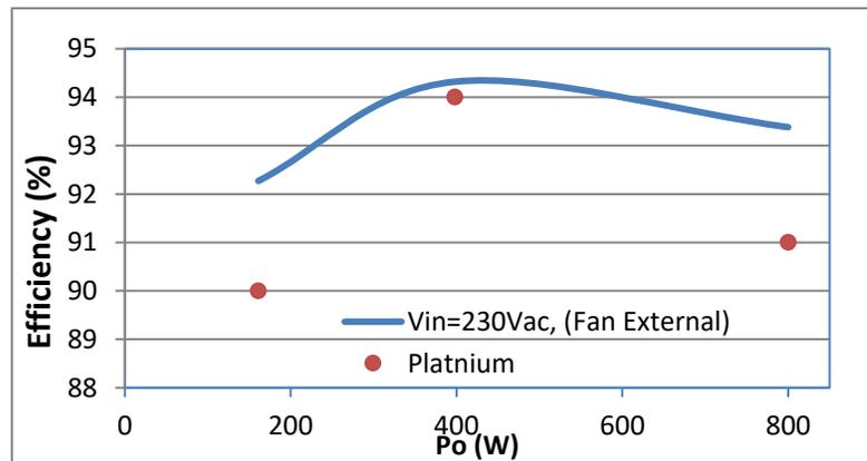
Figure 2. Efficiency vs. Load Current (Ratio Metric Loading)
