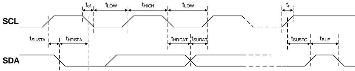
Figure 9. I<sup>2</sup>C / SMBus Timing
