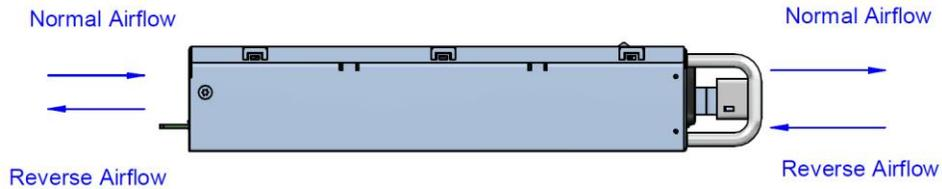
Figure 12. Airflow direction
