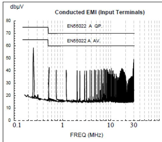
To meet class B for the above standards, it is necessary to fit a 3.3 µF ceramic capacitor across the input terminals.
