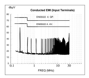
To meet class B for the above standards, it is necessary to fit a 3.3  $\mu\text{F}$  ceramic capacitor across the input terminals.
