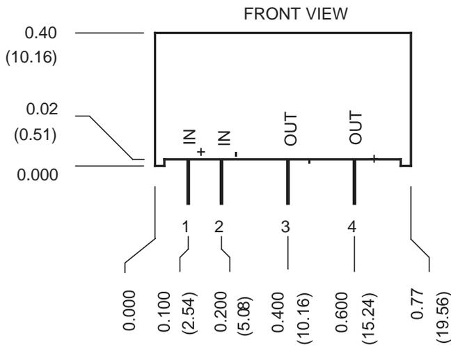
Figure 3. Mechanical Dimensions
