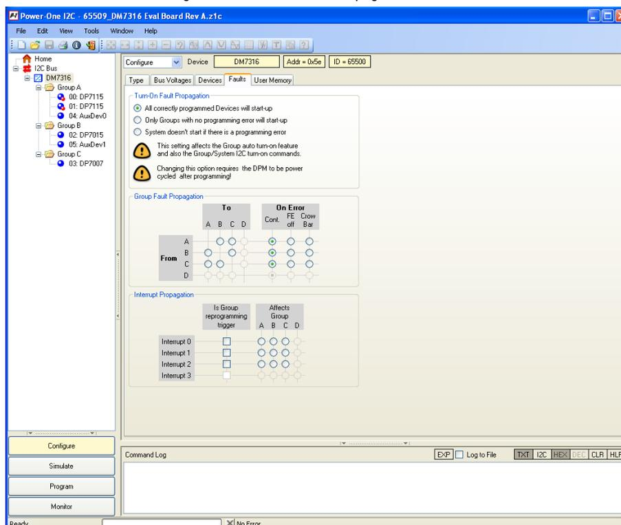
The fault propagation from POL converters to the auxiliary devices can be disabled by checking the bit in the Auxiliary Device Fault Management window as shown in Figure 15. It is not possible to propagate a fault from an Auxiliary Device to POL converters.
