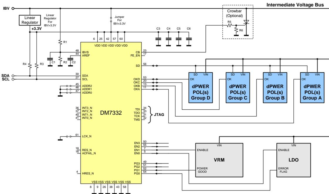
The schematic of a typical application of a DM73XX digital power manager (DPM) is shown in Figure 3. The system includes four groups of d-power Point Of Load converters (POLs). A group is defined as one or more POL converters interconnected via OK pins. Grouping of the POLs enables users to program advanced fault management schemes and define margining functions, monitoring, start-up behavior, and reporting conventions.
