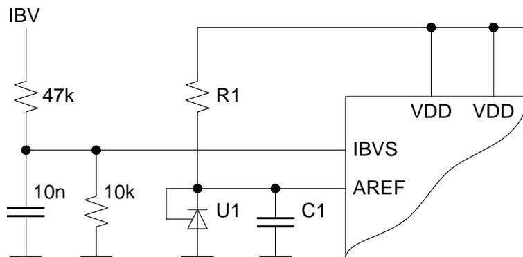
U1 and R1 are additional components. U1 is an industry standard 2.5V voltage reference such as TL431 or similar. C1 is an existing component but its value changes depending on the type of voltage reference. Common voltage reference part numbers and values of associated components are shown in Table 4.
