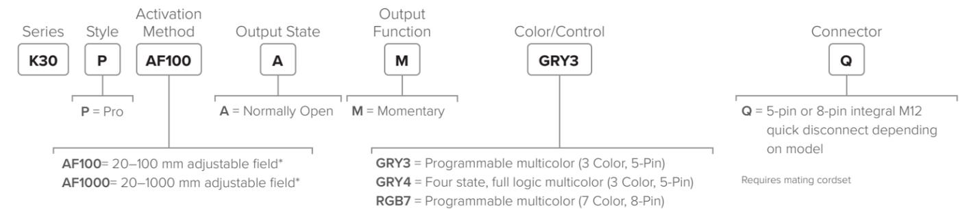
\*Detection distance can be adjusted through teach mode or Pro Editor. Max distance = 1000 mm.
