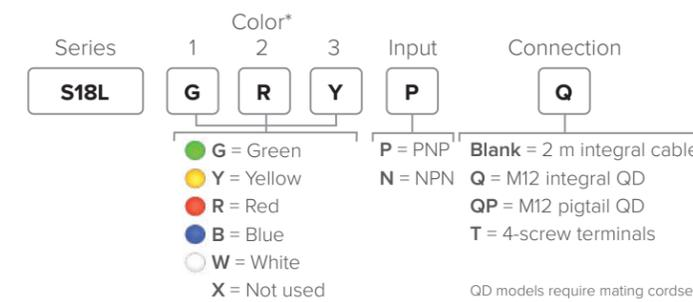
\*Single-color models are available and should be ordered as PNP, but can be wired for either PNP or NPN input
