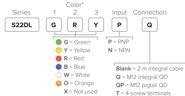
\*Single-color models are available and should be ordered as PNP, but can be wired for either PNP or NPN input
