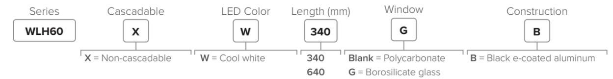
NOTE: Connection for all WLH60 models is a 2 m (6.5') integral FEP cable
