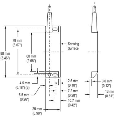
Figure 3. SI-MAG1MM/MM90/MMHF Magnet
