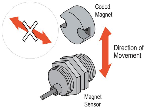
Alternate Direction of Approach: movement is parallel to the plane of the sensing face.
