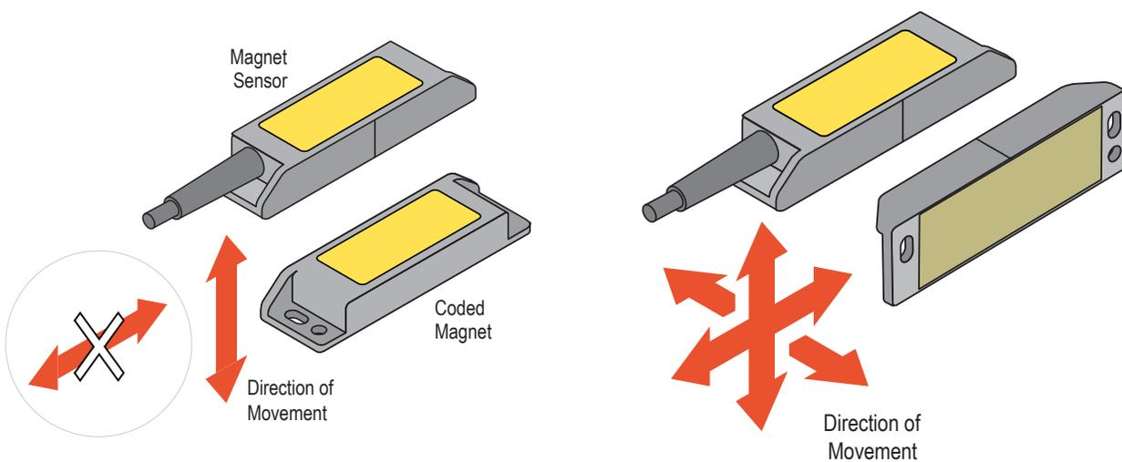
Alternate Direction of Approach: movement is parallel to the plane of the sensing face
