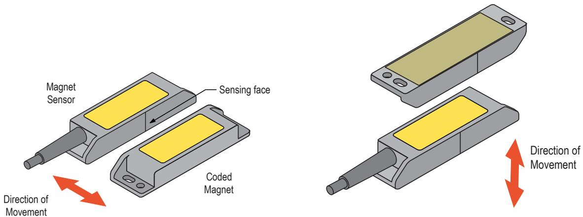
Normal Direction of Approach: movement is perpendicular to the plane of the sensing face
