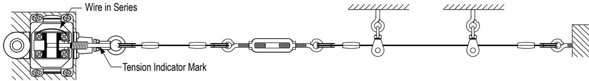
Figure 4. Rope Pulled: Contact 25/26 (45/46) Opens
