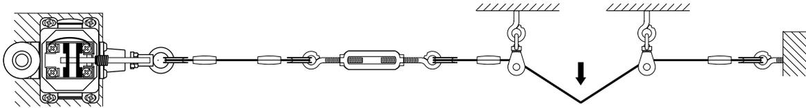
Figure 5. Rope Break or Slack: Contact 13/14 (33/34) Opens
