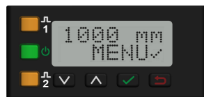
Figure 11. LE550 Display in Run Mode
