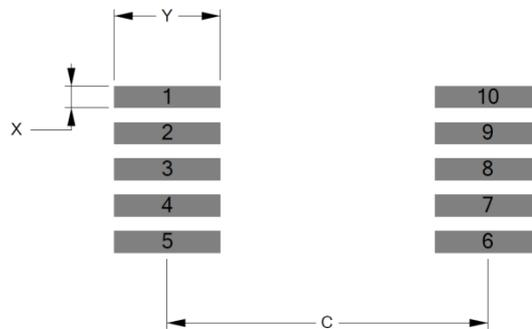
Figure 12.2 MSOP-10 Footprint.
