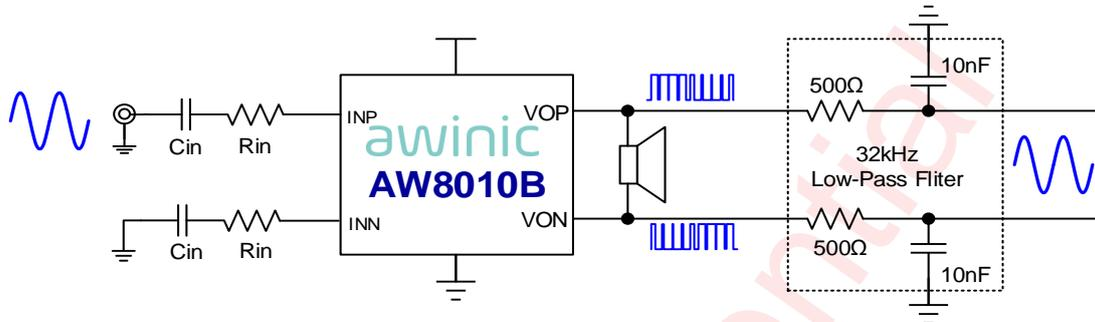
Figure 6 AW8010B test setup
