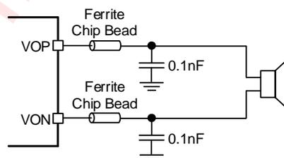
Figure 10 Ferrite Chip Bead and capacitor
