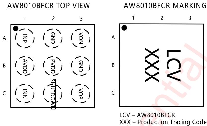
Figure 2 Pin Configuration and Top Mark of AW8010B
