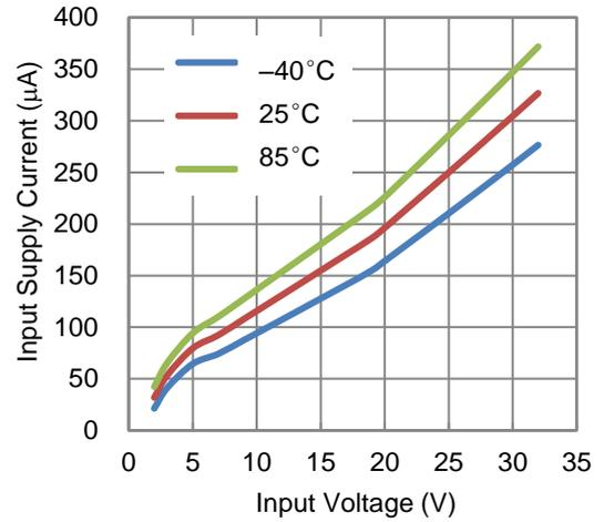
Figure 10 Input Supply Current vs. Supply Voltage
