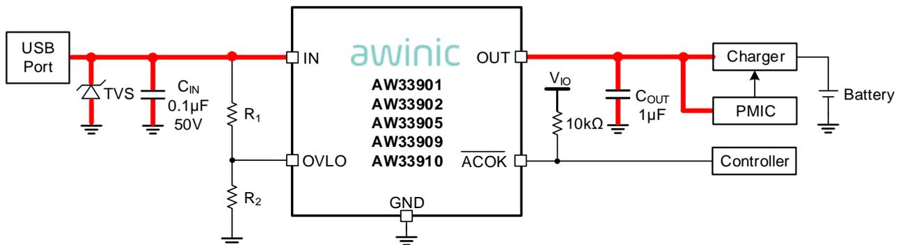
Figure 5 AW339XX typical application circuit(using external OVP threshold)
