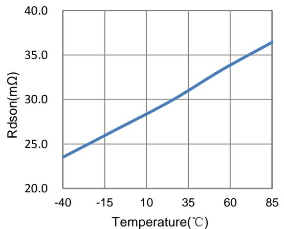
Figure 8  $R_{dson}$  vs. Temp. ( $I_{OUT} = 1A$ )
