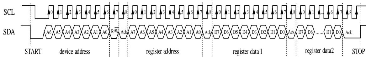
Figure 5 I2C write cycle, multiple registers are written
