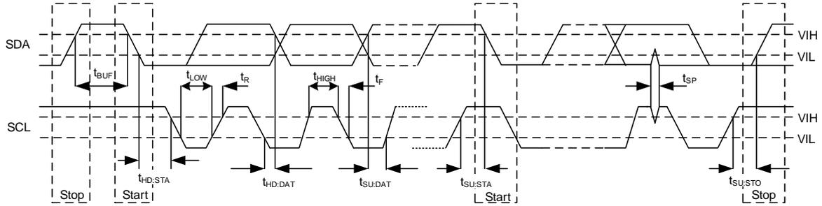
Figure 4 I2C interface timing diagram
