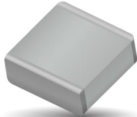
These porcelain and ceramic dielectric multilayer capacitor (MLC) chips are best suited for RF/ Microwave applications typically ranging from 10 MHz to 4.2 GHz. Characteristic is a fine grained, high density, high purity dielectric material impervious to moisture with heavy internal palladium electrodes.
