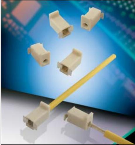
Vertical poke-home connectors were introduced into the market a few years ago to provide a reliable, yet cost effective discrete wire-to-board termination in perpendicular applications. Designed to bridge the gap between inconsistent hand soldering of wires and costly 2-piece connector systems, these connectors are available in a range of positions and configurations while accepting 18 to 26AWG solid or stranded wires.
