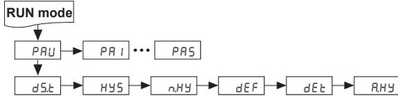
The above is setting user parameter group in the DAQMaster with delay display period [d5t] of parameter 1 group, hysteresis [HY5], night mode hysteresis [nHY] of parameter 2 group, defrost method [dEF], defrost time [dEt] of parameter 3 group, alarm output hysteresis [RHJ] of parameter 4 group.
