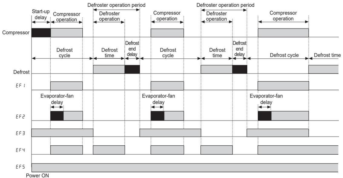
※■: Output does not turn ON but the dedicated indicator flashes at the delay period (compressor, defrost, evaporator-fan).
