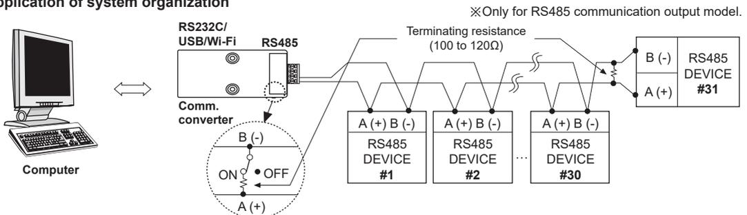
※It is recommended to use Autonics communication converter; SCM-WF48 (Wi-Fi to RS485·USB wireless communication converter, sold separately), SCM-US48I (USB to RS485 converter, sold separately), SCM-38I (RS232C to RS485 converter, sold separately).
