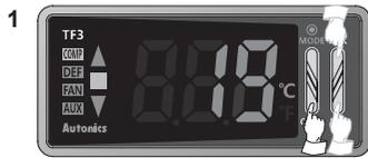
Press any key among the  $\leftarrow$ ,  $\downarrow$ ,  $\rightarrow$  in RUN mode to enter into SV setting mode. Last digit ( $10^0$  digit) on SV display part flashes.
