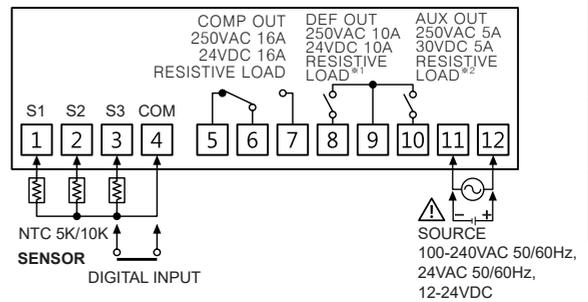
※1: Only for compressor+defrost or auxiliary (alarm/evaporator-fan) output model (TF3□-2□□-□), compressor+defrost+auxiliary (alarm/evaporator-fan) output model (TF3□-3□□-□).
