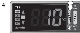
Press the  $\odot$  (MODE) key to save the set value. (If there is no additional key operations in 3 sec, the changed SV is automatically saved.)
