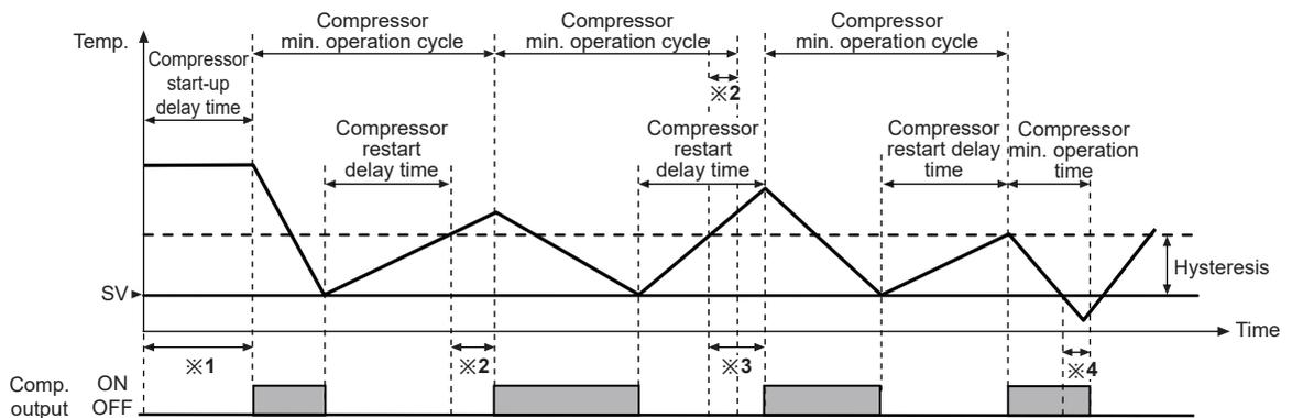
※1: When starting compressor, if present value (PV) is out of hysteresis range, compressor output does not turn ON and the compressor (COMP) output indicator is flashing during compressor start-up delay time.
