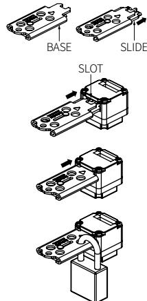
1. Push the SLIDE of the group locking device forward in the direction.
