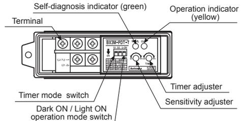
※There are no timer mode switch and the timer adjuster in no timer function type.
