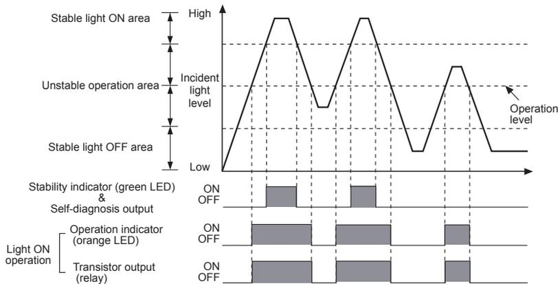
※ The waveforms of "Operation indicator" and "Transistor output" are for Light ON operation. They are opposite operation for Dark ON operation.
