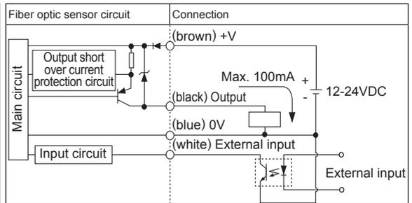
※When using external input function, use photocoupler, external controller, etc. Otherwise, it may result in product damage.
