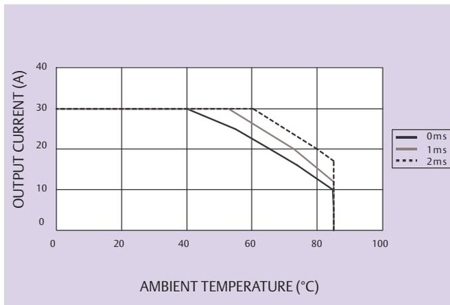
**Figure 3 - Derating Curve**
