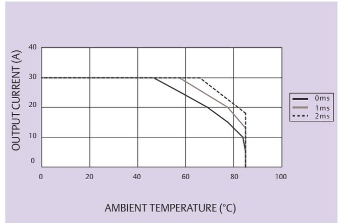
**Figure 2 - Derating Curve**
