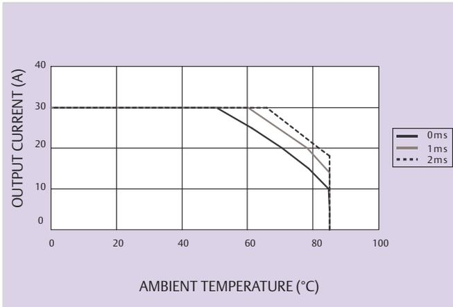
**Figure 1 - Derating Curve**
