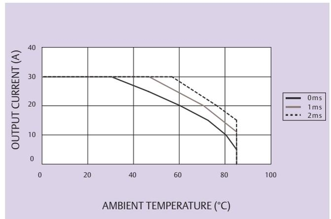
**Figure 4 - Derating Curve**
