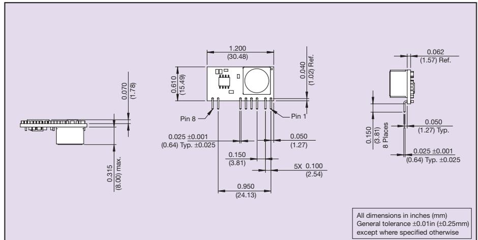
Figure 2: Mechanical Drawing - Vertical Mount Version
