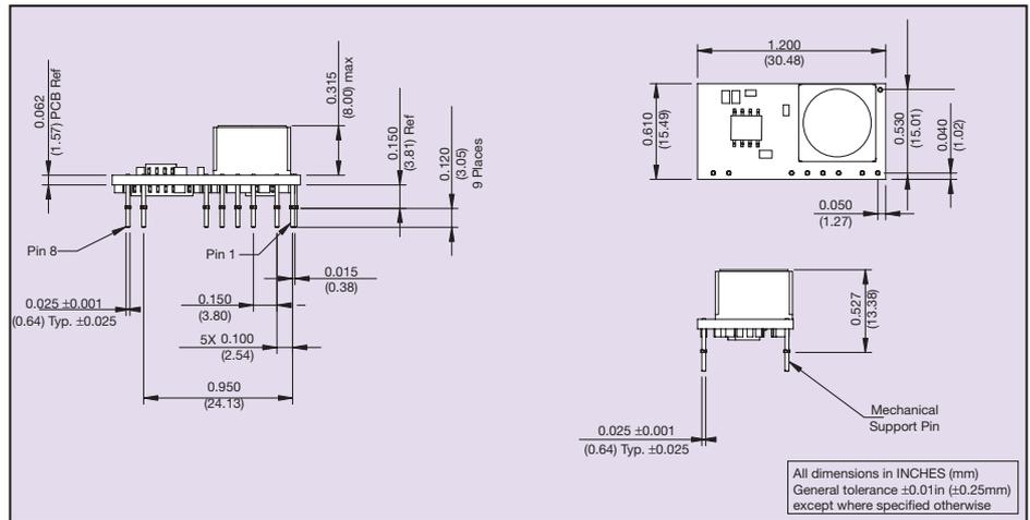
Figure 1: Mechanical Drawing - Horizontal Mount Version
