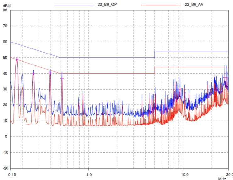
The PSE1000PFC and PSE1000DCDC-12V power supplies with external EMI filters before PSE1000PFC to ensure the converters' conducted EMI levels comply with EN55022 (FCC Part 15) Class B and EN55022 (CISPR 22) Class B limits. The EMI measurements are performed with resistive loads at maximum rated loading.
