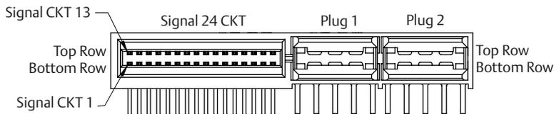
\*Note: The top side of the PSU Output Connector connects with the Bottom Row of the Mating Connector
