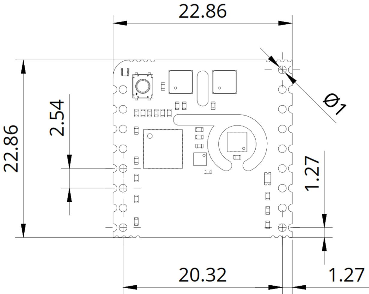
The Nicla Sense Env does not have mounting holes for mechanical fixing. The slots found in the board were placed because of the board's sensor requirements and specifications.
