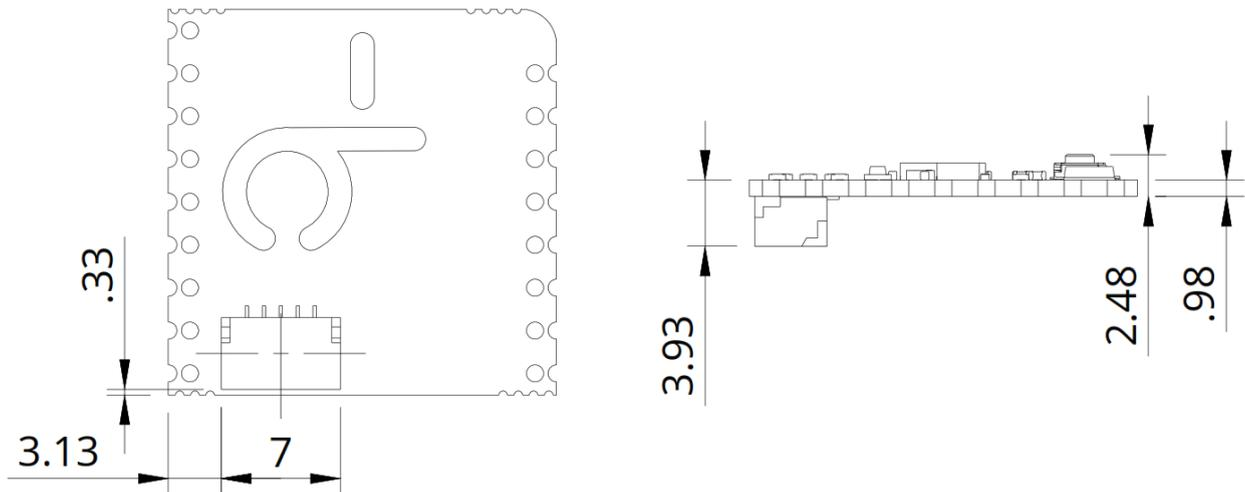
The Nicla Sense Env was designed to be usable as a surface-mount module and presents a dual inline package (DIP) format with the MKR-styled header connectors on a 2.54 mm pitch grid with 1 mm holes.
